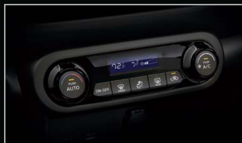
Automatic Climate Control Air-Conditioning
