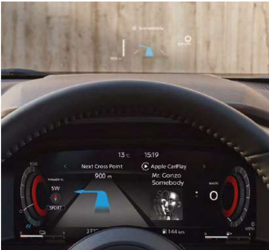
12.3" Fully Digital meter 10.8" Windscreen Head-up display
