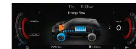
Digital combimeter with energy flow
